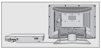
Connect the »AV2« or »AV3« sockets on the television and the corresponding sockets of the video recorder, DVD player or the set-top box with a Euro-AV (Scart) cable.
